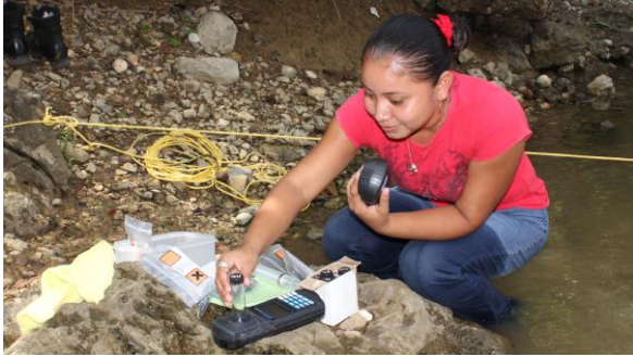
Image 5. Devina Bol testing nitrate levels at site | Image 6. Octavio testing for Dissolve Oxygen
