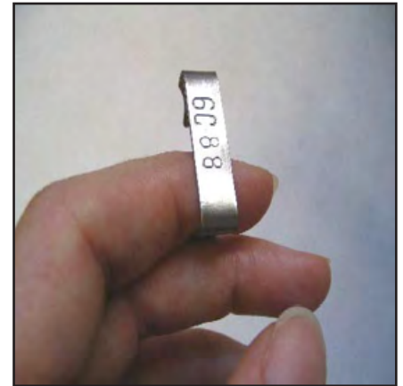
Figure 1: Hold a flipper tag in correct orientation to load into applicator. Note that the number side of the tag is up.
