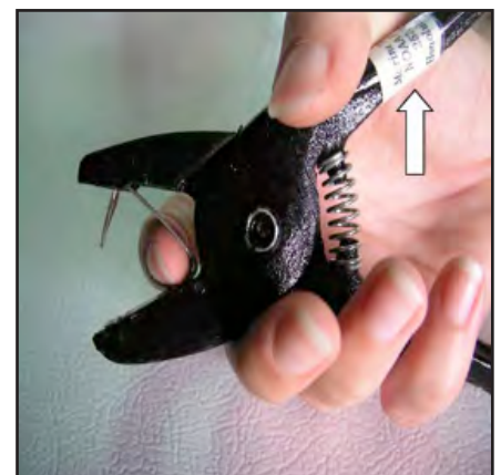
Figure 2: A fully seated tag in the tag applicator pliers.
